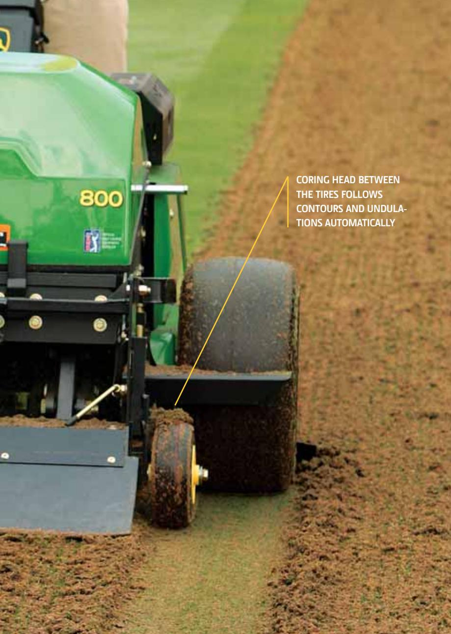
CORING HEAD BETWEEN THE TIRES FOLLOWS CONTOURS AND UNDULATIONS AUTOMATICALLY
