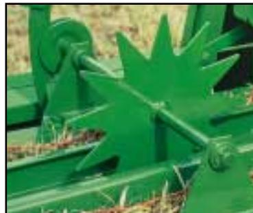
*The centre mounted measuring wheel provides a consistent and accurate measurement of the bale length. Adjust the bale length to meet your needs (from 0.3 m to 1.3 m). Fast speeds? Rough Terrain? The adjustable arm securely locks in place enhanced accuracy in these tough conditions.*
