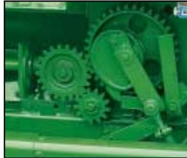
*John Deere gear driven knotters run like clockwork. There are no chains in this system to oil or adjust. Timing problems are eliminated. Heavy needle lift shafts deliver long lasting performance.*
