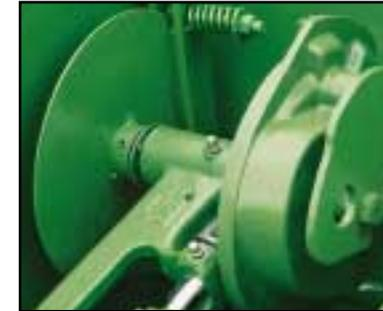
*The needle brake facings maintain a constant force to keep the needle out of the balecase after the tying cycle, even in the roughest terrain, and prevent backslap. The brake is designed for durability and a long service life.*
