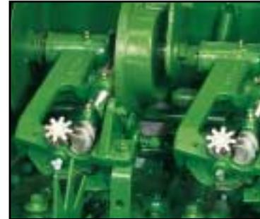
*Needles, made of formed steel for long life, bring twine to the knotters after each cycle of the measuring wheel. And surgical quality steel twine knives are easily removed for sharpening or replacement.*
