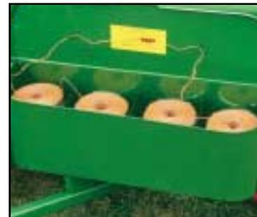
*Twine box – Models 349 and 359. Load up with an all-day supply of twine. You spend less time refilling and more time baling. The twine box is completely enclosed. Refilling is made quick and easy.*
