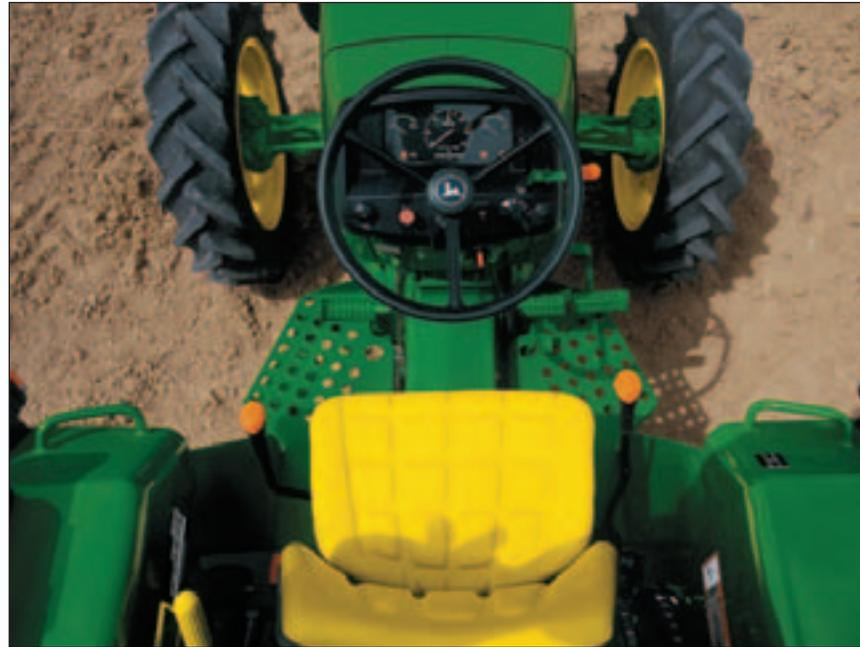
The driver has an easy and comfortable drive with the wide, flat driving platform. And the adjustable suspension driver's seat ensures comfort for long periods of time. There are no controls in the foot area in the driver's platform to obstruct legs or cause discomfort to the driver.
