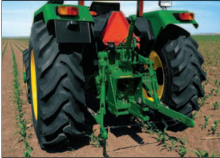
*With its three-point hydraulic suspension system, it has the lifting capacity for any lifting requirement, even the heaviest. And when working with compatible equipment, high performance, comfort and safety are guaranteed with its independent PTO.*
